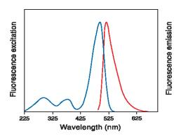
Figure 1. Excitation (blue) and emission spectra (red) of **SYBR Green I** bound to dsDNA in TBE buffer.
